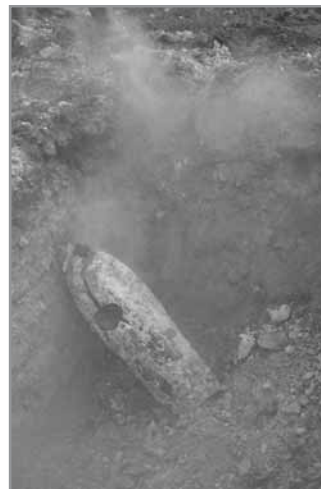
Figure 2.5 C50A phosphorus incendiary bomb that had only partially functioned, reigniting after exposure to air
